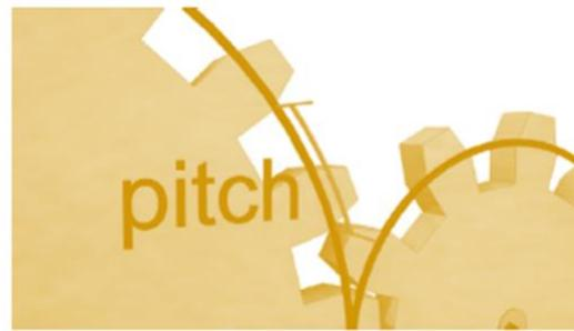
During laboratory work, students conclude that a pair of gears may have different radii to gearing, but must have the same tooth pitch.
